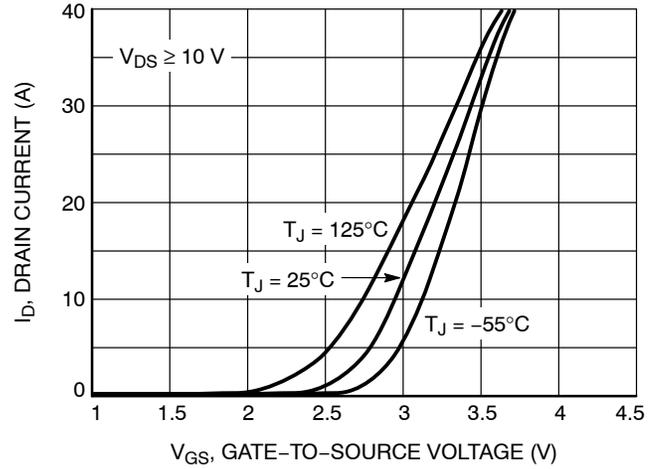
Figure 2. Transfer Characteristics
