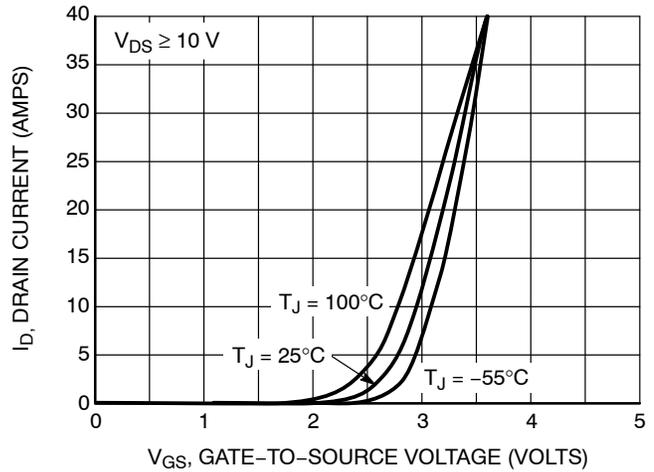
Figure 2. Transfer Characteristics
