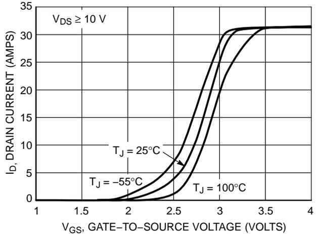
Figure 2. Transfer Characteristics
