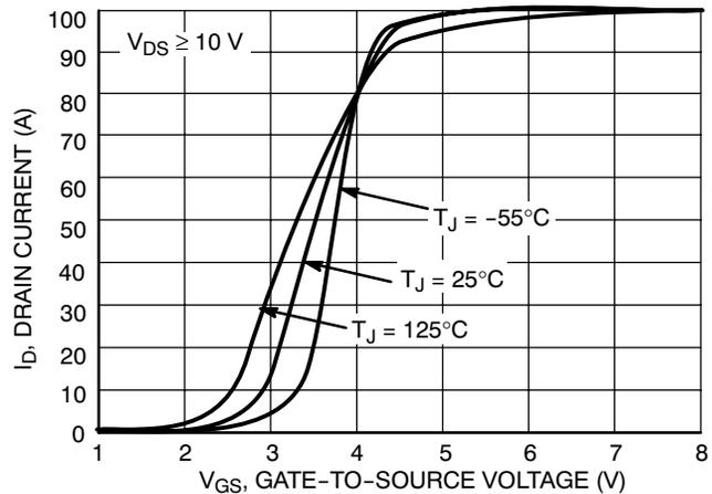
Figure 2. Transfer Characteristics
