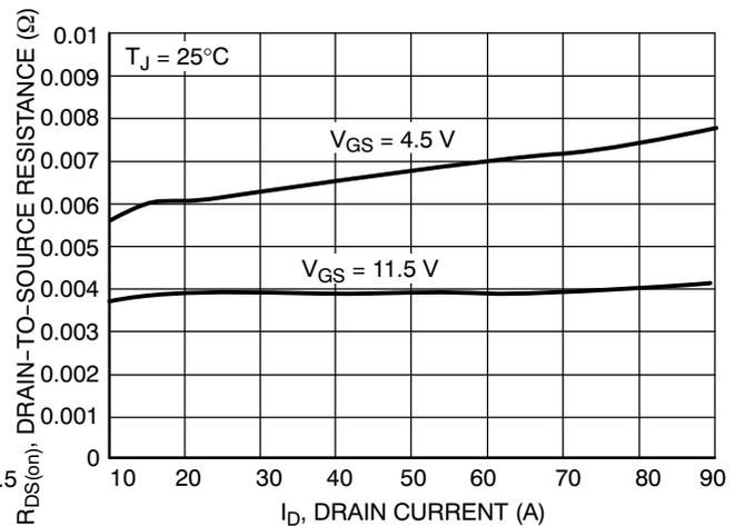
Figure 4. On-Resistance vs. Drain Current & Gate Voltage
