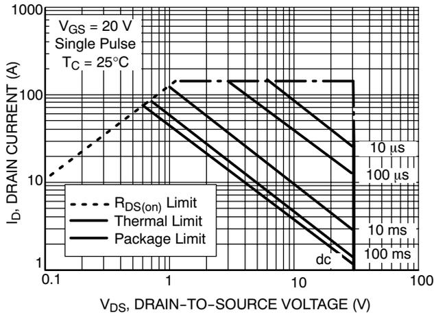
**Figure 11. Maximum Rated Forward-Biased Safe Operating Range**
