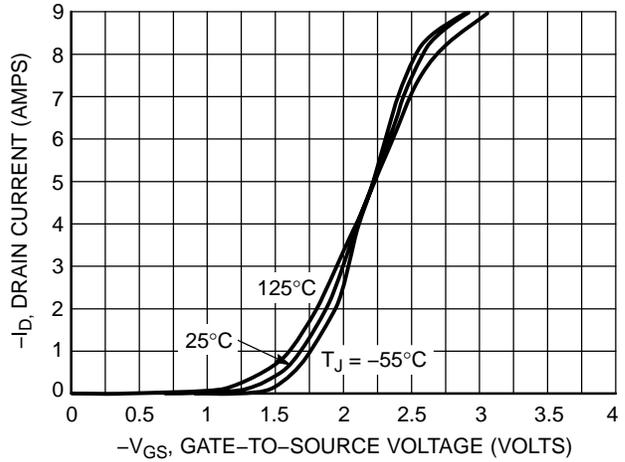
Figure 2. Transfer Characteristics
