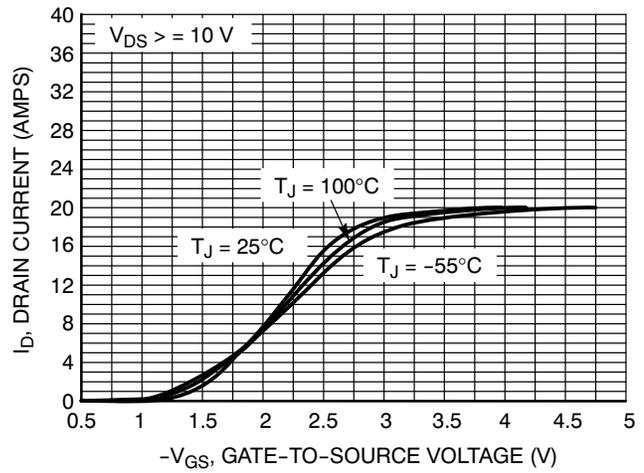
**Figure 2. Transfer Characteristics**
