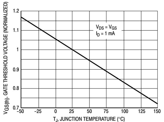
Figure 6. Gate Threshold Voltage Variation with Temperature
