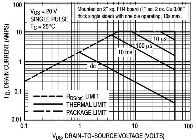
Figure 9. Maximum Rated Forward Biased Safe Operating Area
