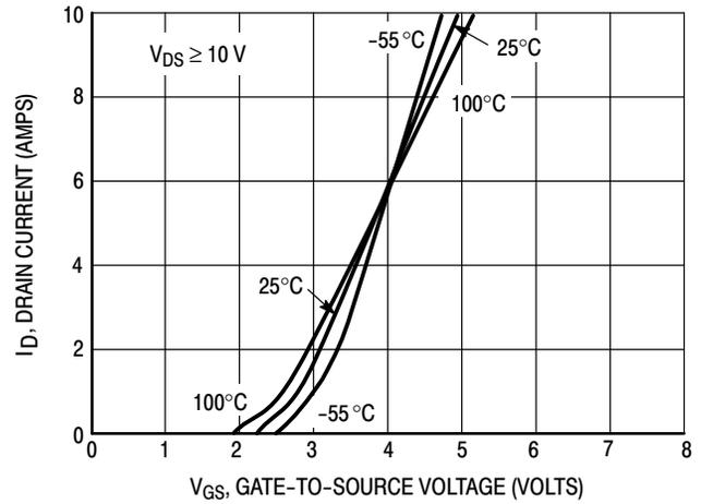
Figure 2. Transfer Characteristics
