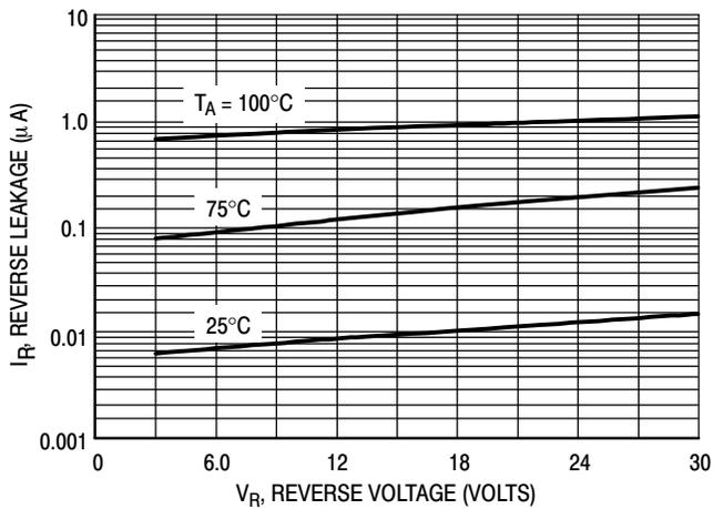
Figure 3. Reverse Leakage
