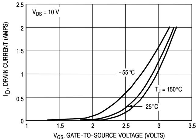
Figure 1. Transfer Characteristics
