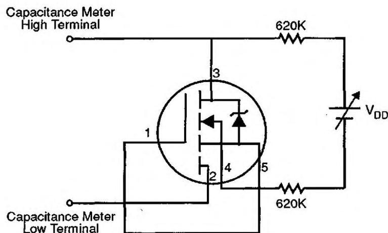
**Fig 19.** HEXSense Sensing Cell Output Capacitance Test Circuit
