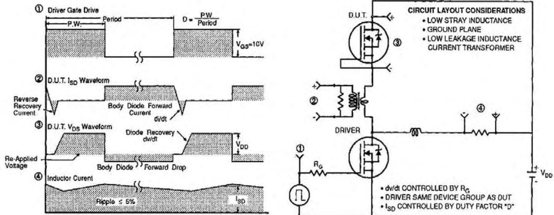
Fig 14. Peak Diode Recovery dv/dt Test Circuit
