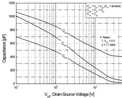
Figure 5. Capacitance Characteristics
