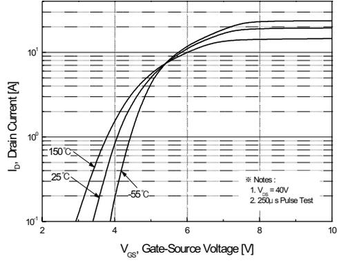
Figure 2. Transfer Characteristics
