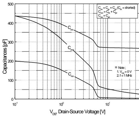
Figure 5. Capacitance Characteristics
