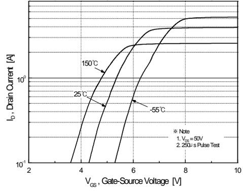
Figure 2. Transfer Characteristics
