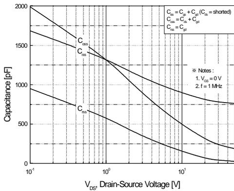
**Figure 5. Capacitance Characteristics**
