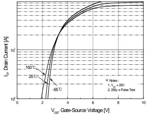
**Figure 2. Transfer Characteristics**
