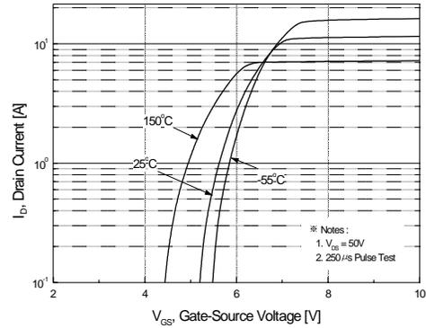
Figure 2. Transfer Characteristics
