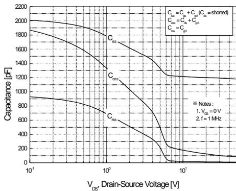
Figure 5. Capacitance Characteristics
