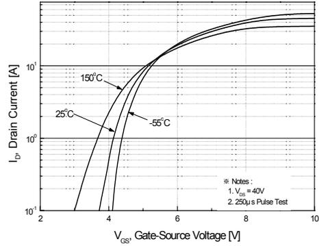
Figure 2. Transfer Characteristics
