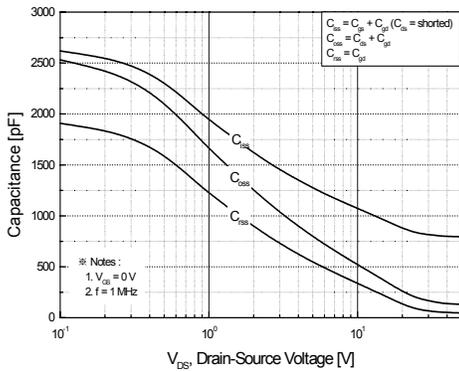
Figure 5. Capacitance Characteristics
