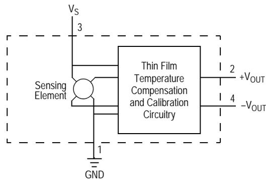
**Figure 1. Temperature Compensated and Calibrated Pressure Sensor Schematic**
