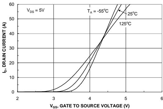
Figure 5. Transfer Characteristics.
