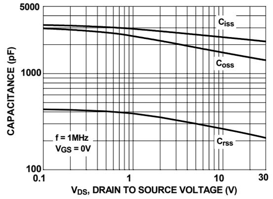
Figure 19. Capacitance vs Drain to Source Voltage
