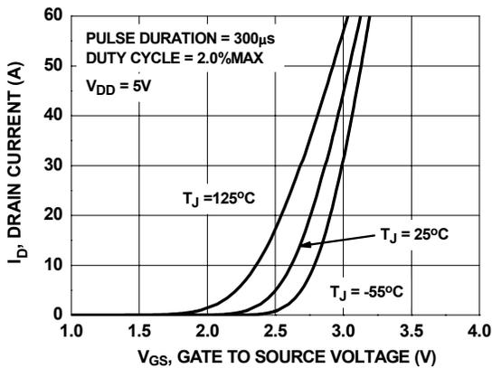
Figure 16. Transfer Characteristics
