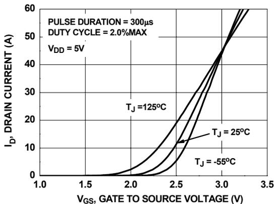
Figure 5. Transfer Characteristics
