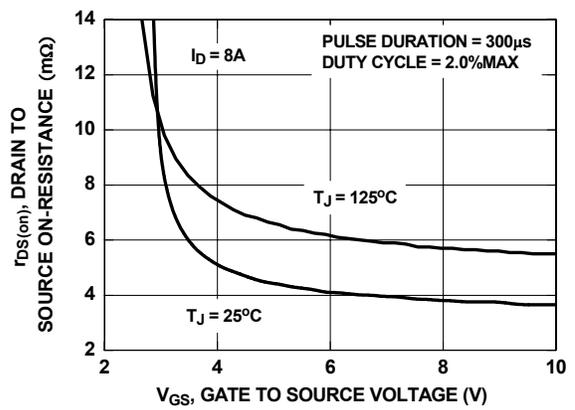
Figure 15. On-Resistance vs Gate to Source Voltage
