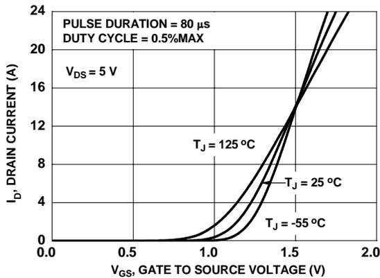
**Figure 5. Transfer Characteristics**
