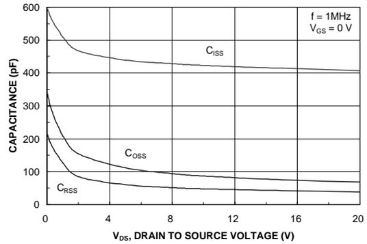
Figure 8. Capacitance Characteristics.
