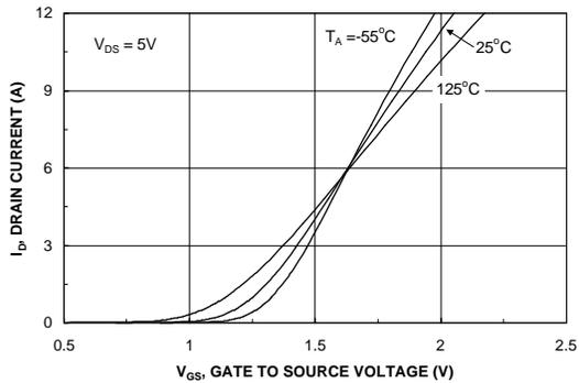
Figure 5. Transfer Characteristics.
