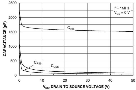
Figure 8. Capacitance Characteristics.
