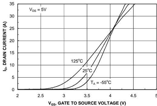
Figure 5. Transfer Characteristics.
