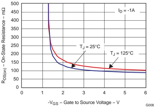
Figure 6. On-State Resistance vs. Gate Voltage
