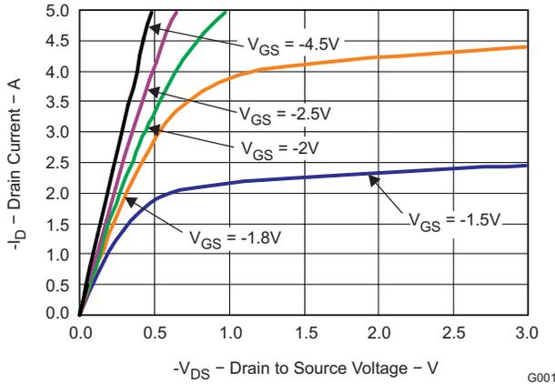
Figure 2. Saturation Characteristics
