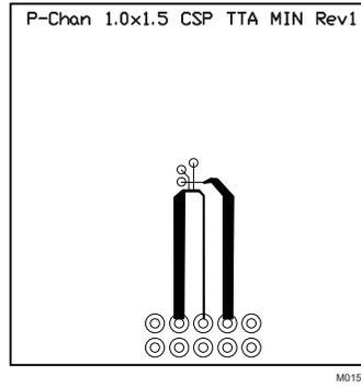
Max  $R_{\theta JA} = 212^{\circ}\text{C/W}$
