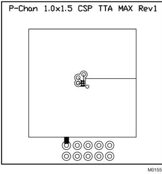
Max  $R_{\theta JA} = 119^{\circ}\text{C/W}$
