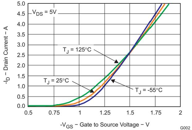
Figure 3. Transfer Characteristics
