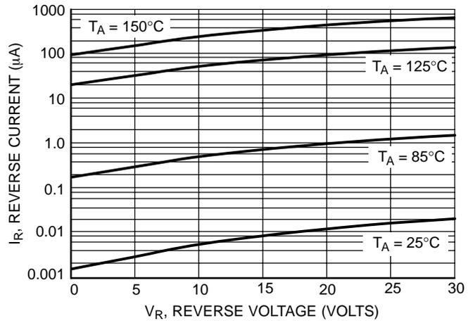
**Figure 3. Leakage Current**
