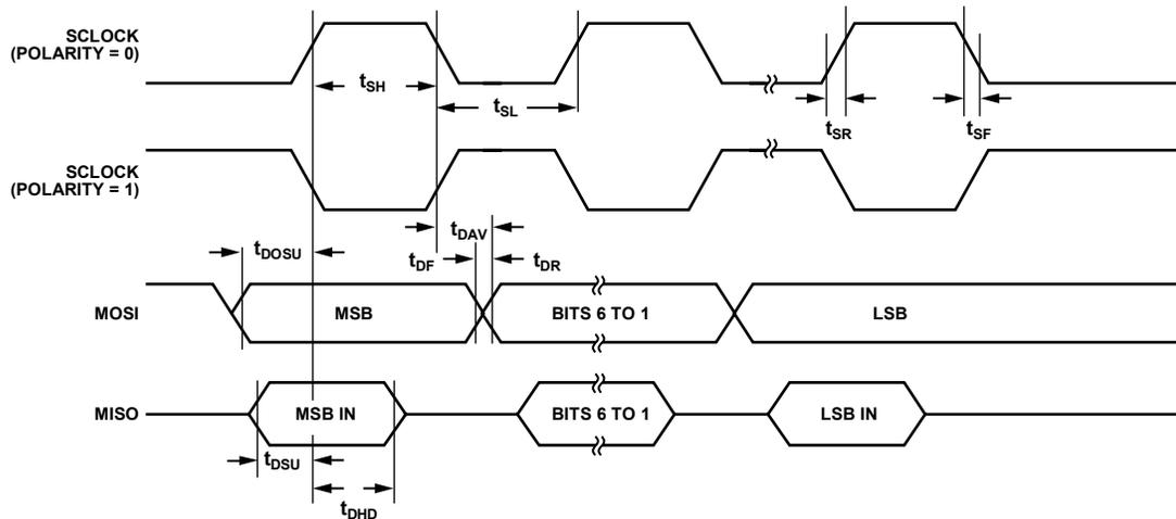
Figure 7. SPI Master Mode Timing (PHASE Mode = 0)
