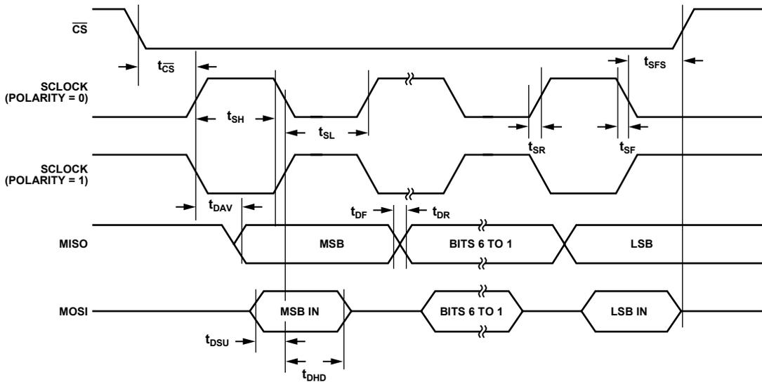
Figure 8. SPI Slave Mode Timing (PHASE Mode = 1)
