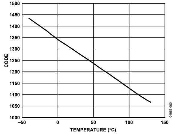
Figure 27. On-Chip Temperature Sensor Voltage Output vs. Temperature
