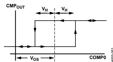
Figure 55. Comparator Hysteresis Transfer Function
