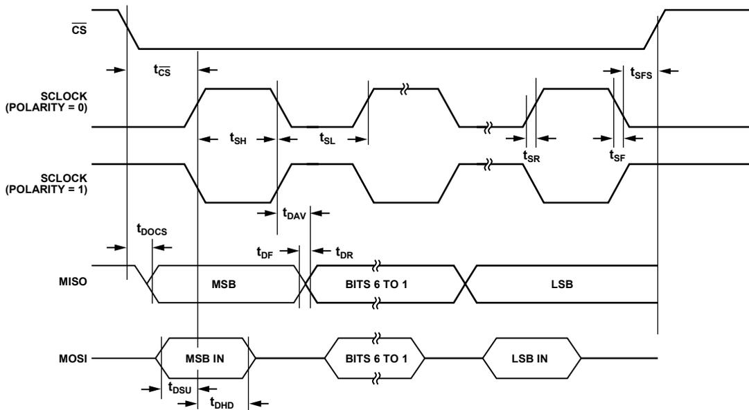
Figure 9. SPI Slave Mode Timing (PHASE Mode = 0)
