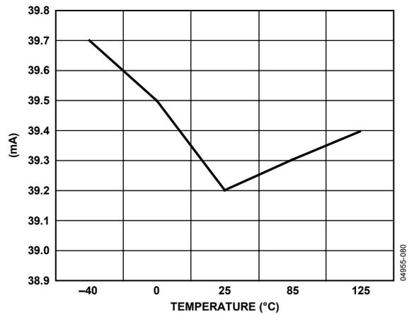
Figure 28. Current Consumption vs. Temperature @  $CD = 0$
