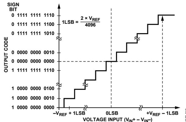
Figure 39. ADC Transfer Function in Differential Mode
