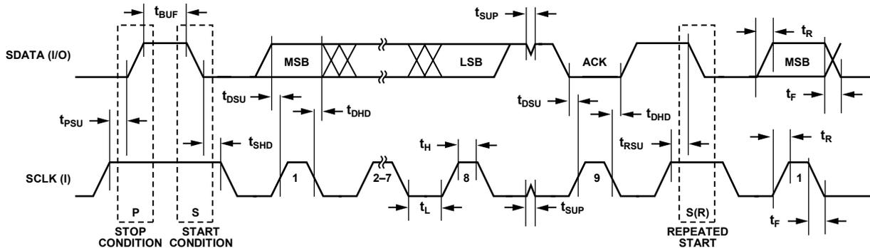
Figure 5. I<sup>2</sup>C Compatible Interface Timing
