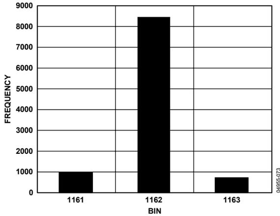
Figure 23. Code Histogram Plot,  $f_s = 774$  kSPS,  $V_{IN} = 0.7$  V
