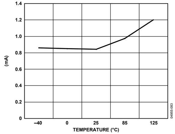
Figure 31. Current Consumption vs. Temperature in Sleep Mode
