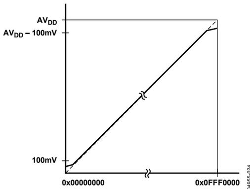
Figure 53. Endpoint Nonlinearities Due to Amplifier Saturation
