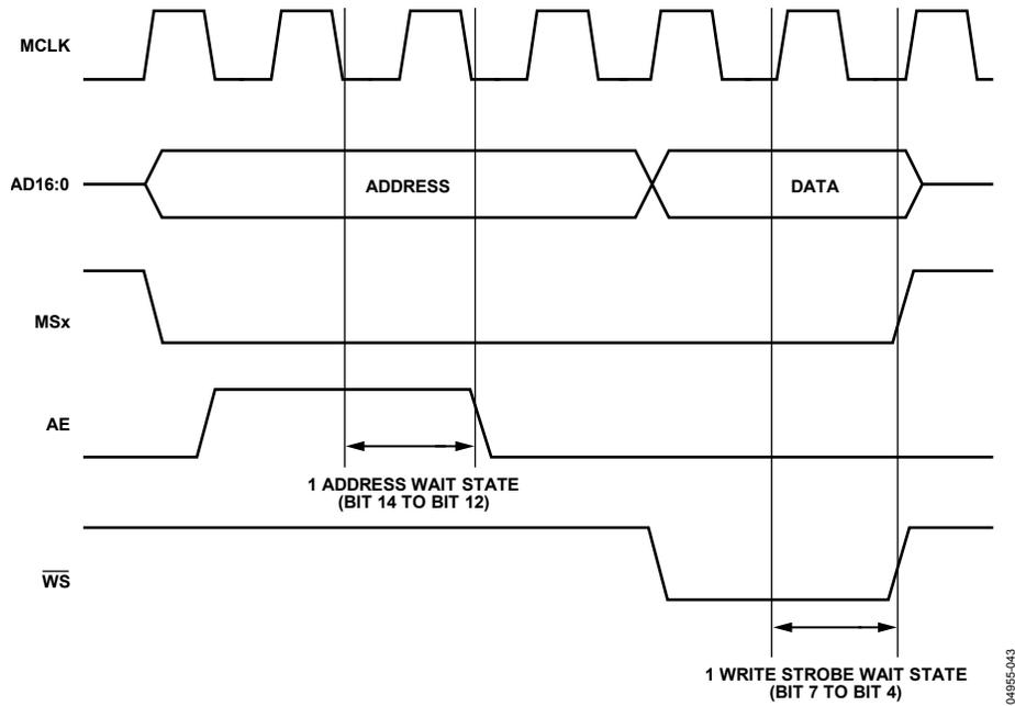
Figure 73. External Memory Write Cycle with Wait States
