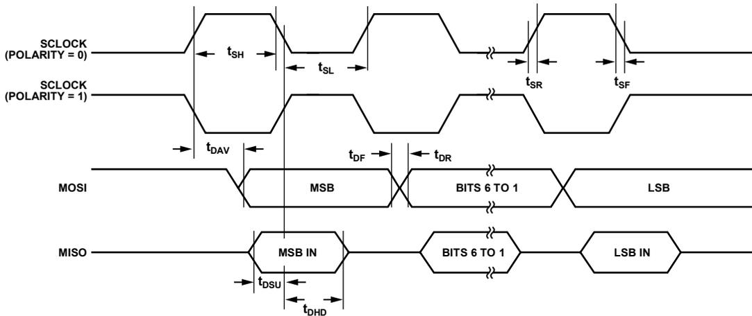
Figure 6. SPI Master Mode Timing (PHASE Mode = 1)
