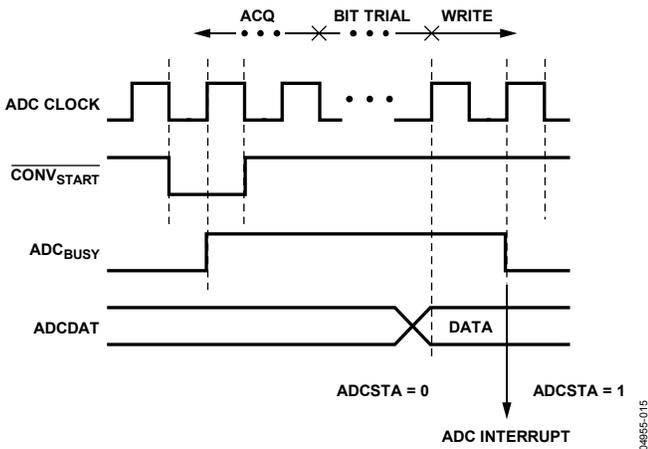
Figure 41. ADC Timing
