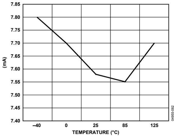
Figure 30. Current Consumption vs. Temperature @ CD = 7
