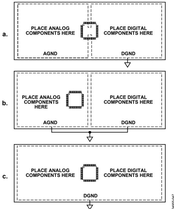
Figure 78. System Grounding Schemes
