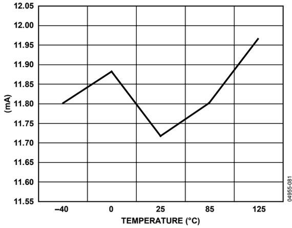
Figure 29. Current Consumption vs. Temperature @ CD = 3
