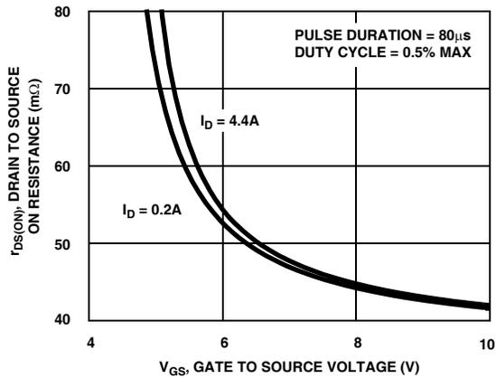
**Figure 3. On-Resistance vs Gate to Source Voltage**
