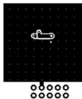
a.  $60^\circ\text{C}/\text{W}$  when mounted on a 1 in<sup>2</sup> pad of 2 oz copper
