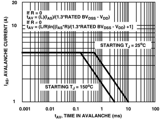
**Figure 8. Uncalamped Inductive Switching Capability**
