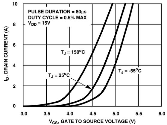
**Figure 4. Transfer Characteristics**
