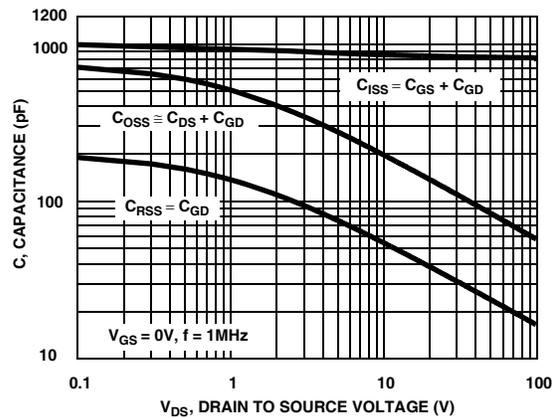
**Figure 6. Capacitance vs Drain to Source Voltage**
