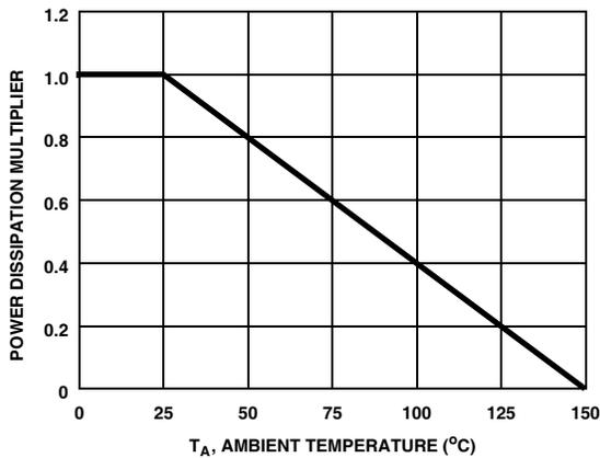
**Figure 9. Normalized Power dissipation vs Ambient Temperature**
