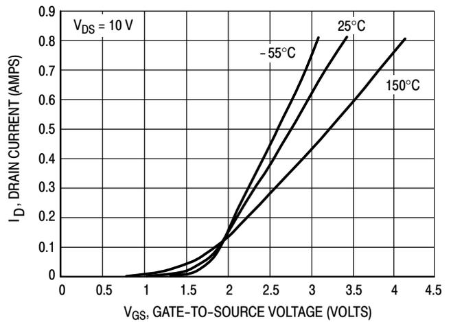
Figure 2. Transfer Characteristics
