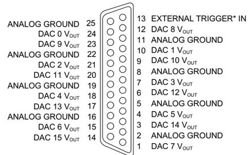
Figure 2. Analog Output Channel Connector - P3
