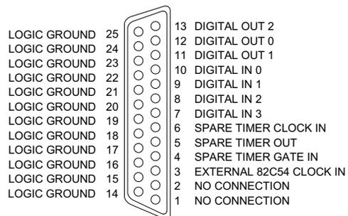
Figure 3. Digital I/O Connector - P4
