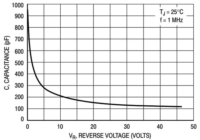
Figure 12. Typical Capacitance
