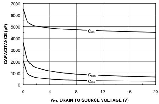
**Figure 8. Capacitance Characteristics.**
