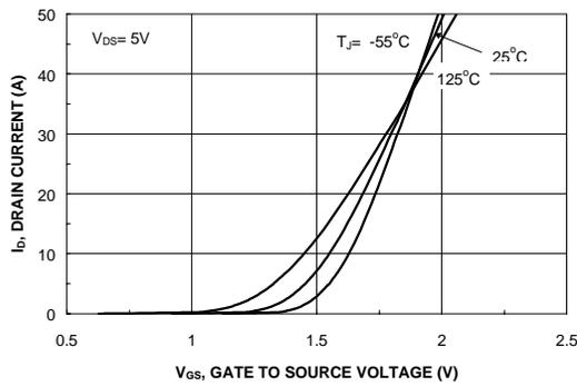
**Figure 5. Transfer Characteristics.**
