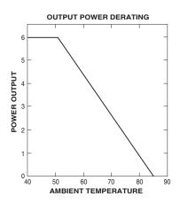
Typical Performance: (Tc=25°C, Vin=Nom VDC, Rated Load)
