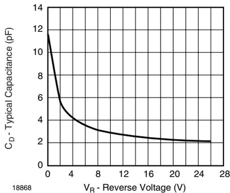
Figure 2. Typical Capacitance  $^{\circ}\text{C}$  vs. Reverse Applied Voltage  $V_R$
