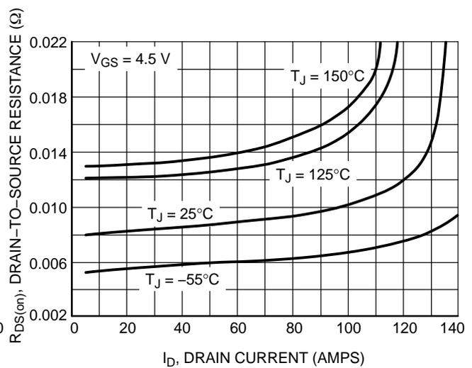
Figure 4. On-Resistance versus Drain Current and Temperature
