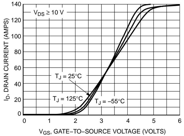
Figure 2. Transfer Characteristics
