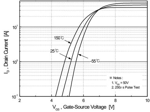
Figure 2. Transfer Characteristics
