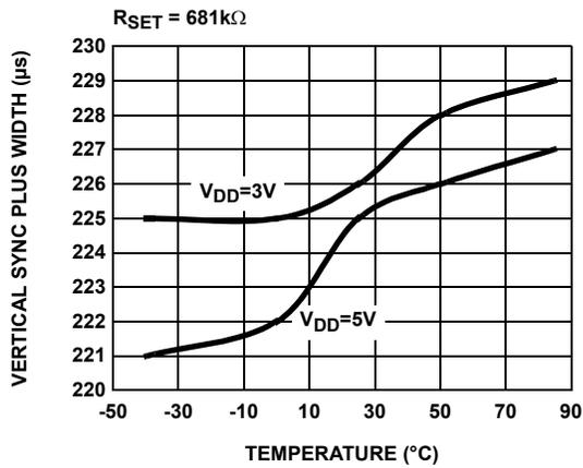
FIGURE 9. VERTICAL SYNC PULSE WIDTH vs TEMPERATURE
