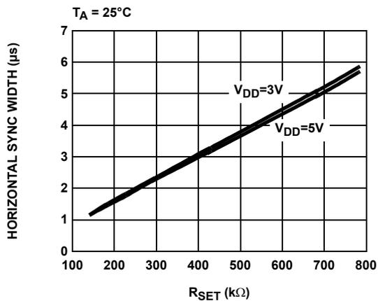
FIGURE 3. HORIZONTAL SYNC WIDTH vs R<sub>SET</sub>
