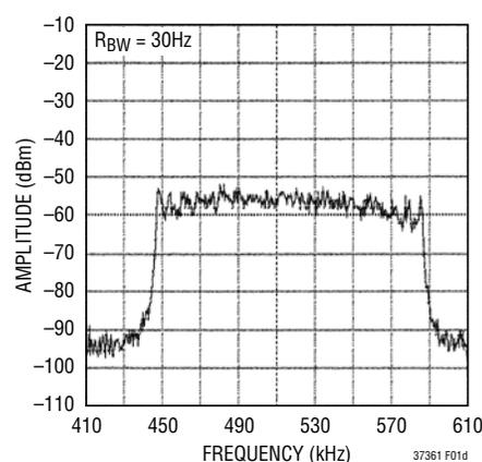
**Figure 1d. Zoom-In of Fundamental Frequency of the LTC3776 Spread Spectrum Buck Switching Converter. Note the >20dB Reduction in Peak Amplitude and Spreading of the Frequency Spectrum (Between Approximately 450kHz and 580kHz) Compared to Figure 1b.**
