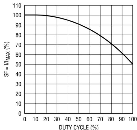
Figure 2. Maximum Peak Current vs Duty Cycle
