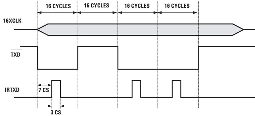
Figure 7. HSDL-7002 Encoding Scheme
