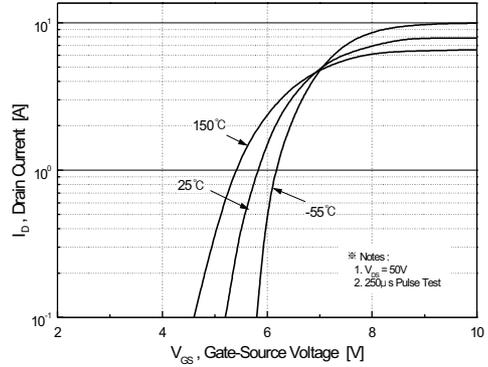
Figure 2. Transfer Characteristics
