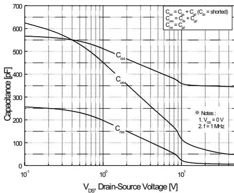
Figure 5. Capacitance Characteristics
