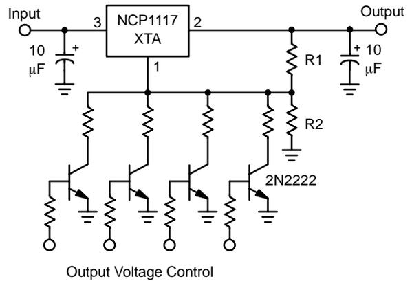
Resistor R2 sets the maximum output voltage. Each transistor reduces the output voltage when turned on.
