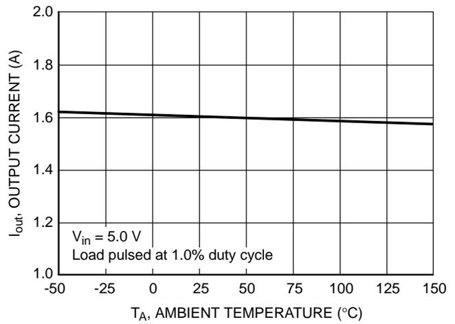
Figure 7. Output Short Circuit Current vs. Temperature
