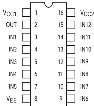
Pin assignment is for Dual-in-Line Package.
