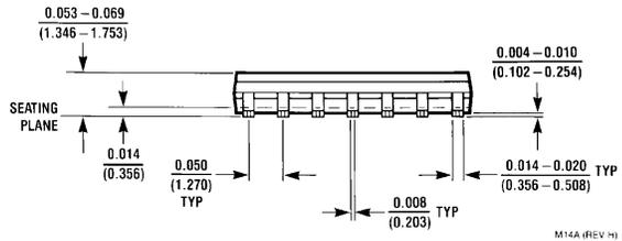
**14-Lead Small Outline Integrated Circuit (SOIC), JEDEC MS-120, 0.150" Narrow Body
