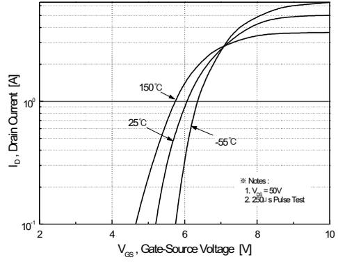
Figure 2. Transfer Characteristics
