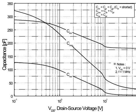
Figure 5. Capacitance Characteristics
