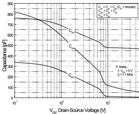
Figure 5. Capacitance Characteristics
