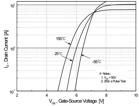
Figure 2. Transfer Characteristics
