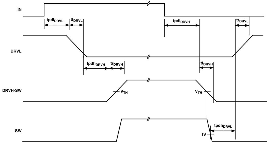
Figure 2. Nonoverlap Timing Diagram
