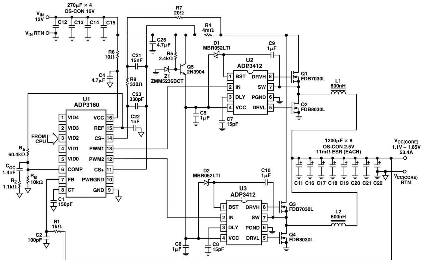
Figure 3. 53.4 A Intel CPU Supply Circuit
