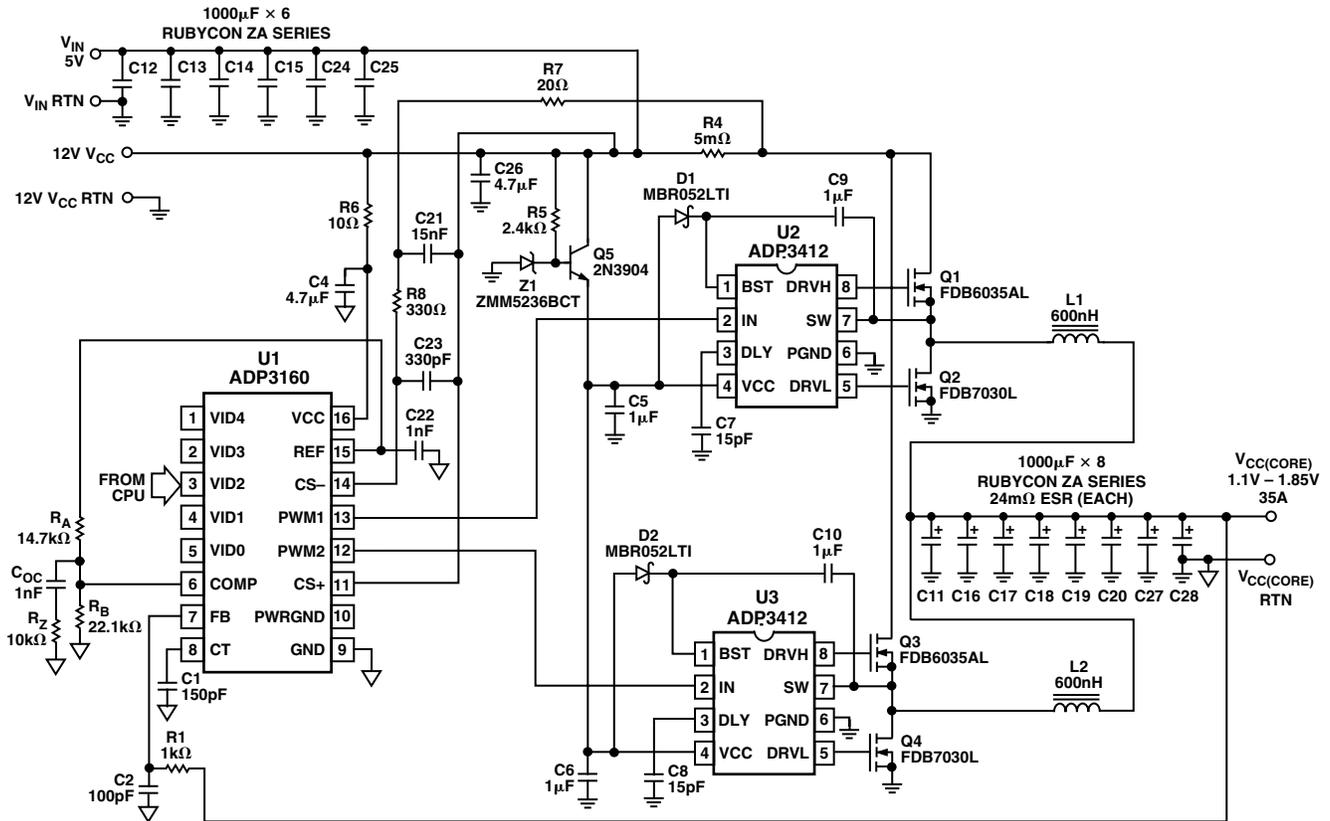
Figure 4. 35 A Athlon CPU Supply Circuit
