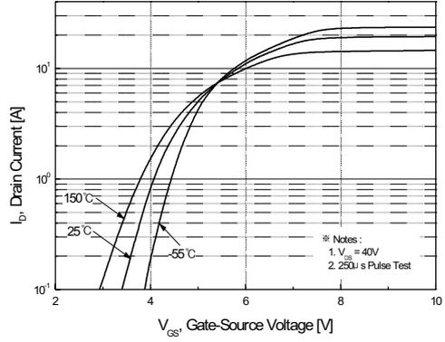
Figure 2. Transfer Characteristics
