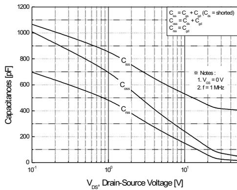
Figure 5. Capacitance Characteristics
