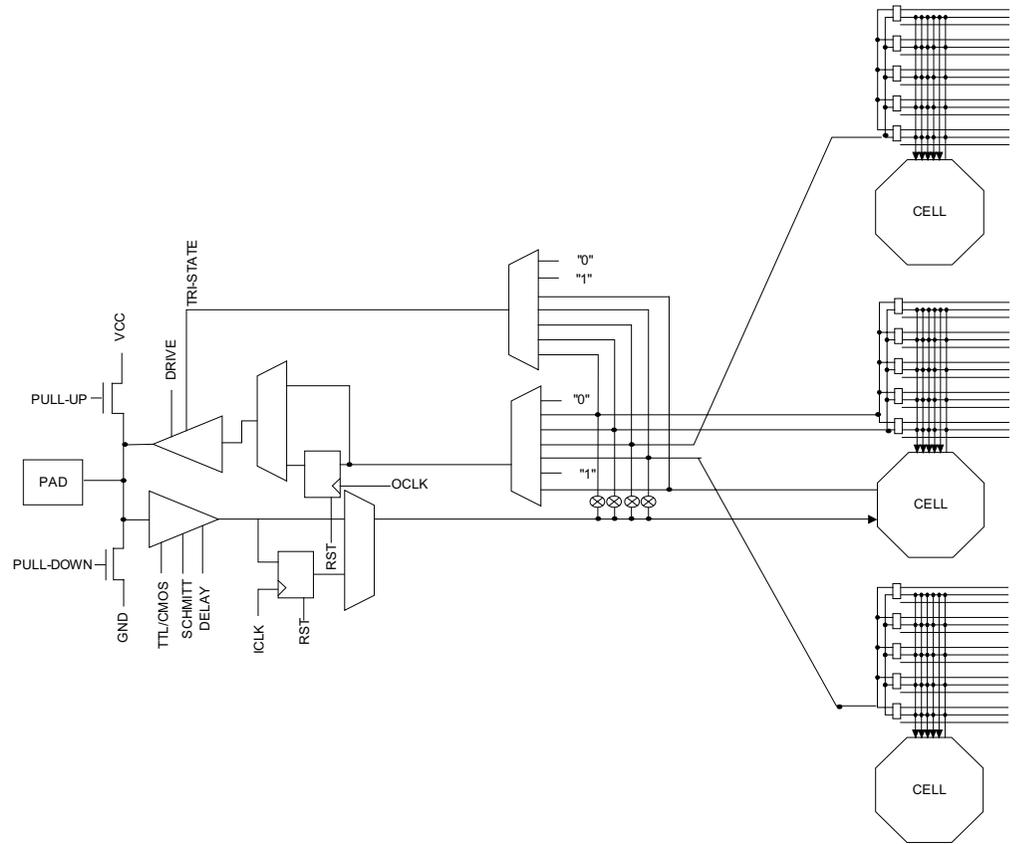
**Figure 13. West Secondary I/O (Mirrored for East I/O)**
