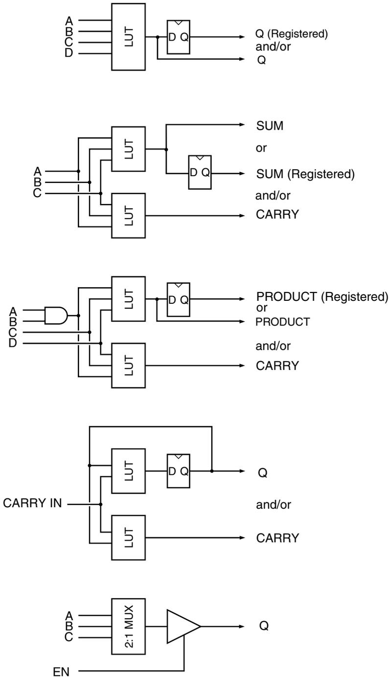
**Synthesis Mode.** This mode is particularly important for the use of VHDL/Verilog design. VHDL/Verilog Synthesis tools generally will produce as their output large amounts of random logic functions. Having a 4-input LUT structure gives efficient random logic optimization without the delays associated with larger LUT structures. The output of any cell may be registered, tri-stated and/or fed back into a core cell.
