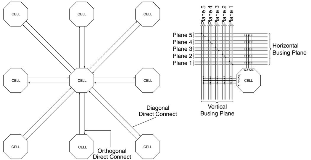
(a) Cell-to-cell Connections
