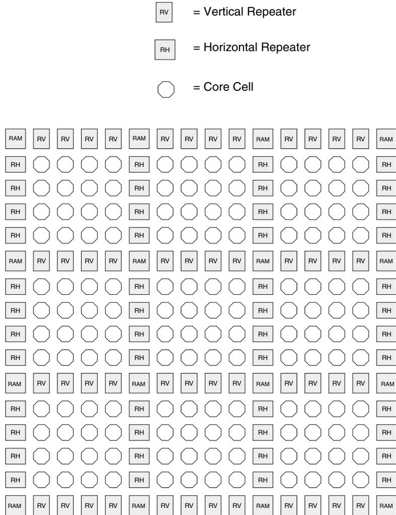
Note: 1. Repeaters regenerate signals and can connect any bus to any other bus (all pathways are legal) on the same plane. Each repeater has connections to two adjacent local-bus segments and two express-bus segments. This is done automatically using the integrated development system (IDS) tool.
