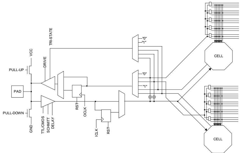
Figure 14. Northwest Corner I/O (Similar NE/SE/SW Corners)
