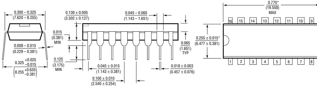
\*THESE DIMENSIONS DO NOT INCLUDE MOLD FLASH OR PROTRUSIONS.
