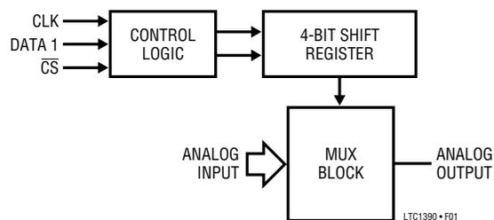
Figure 1: Simplified Block Diagram of the MUX Operation
