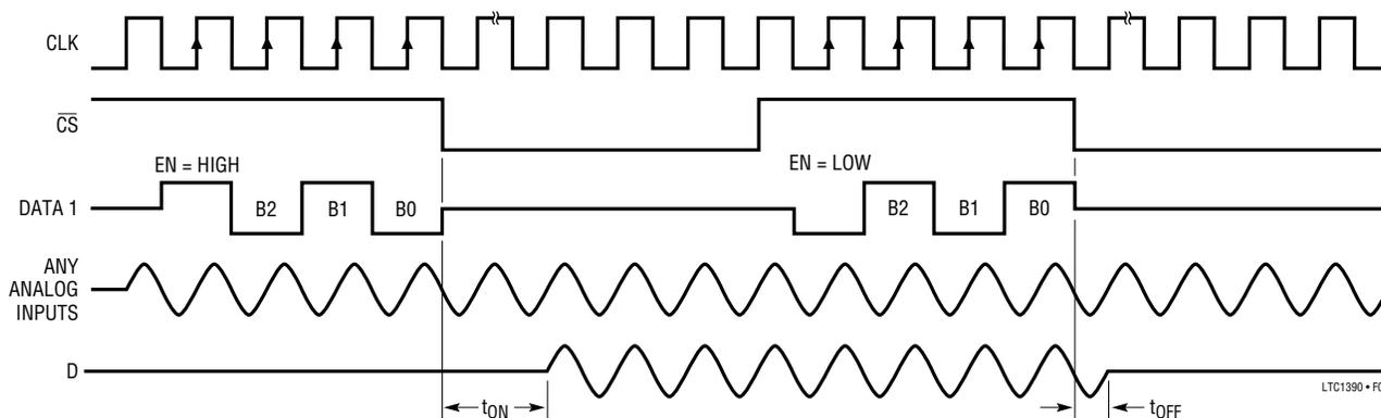
Figure 2: Multiplexer Operation
