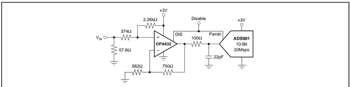
FIGURE 4. DC-Coupled Interface Circuit for  $+3\text{V}$  Single-Supply Operation.
