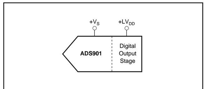
FIGURE 7. Independent Supply Connection for Output Stage.
