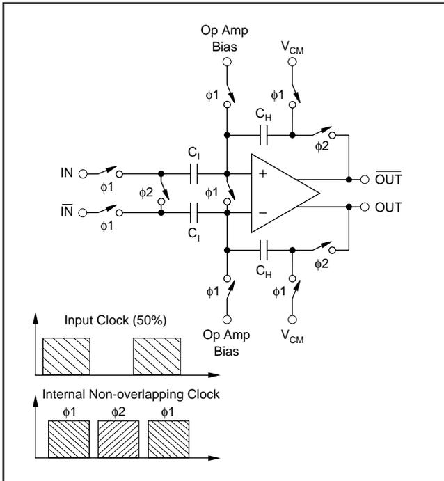
FIGURE 1. Input Track/Hold Configuration with Timing Signals.
