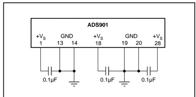
FIGURE 8. Recommended Bypassing for Analog Supply Pins.
