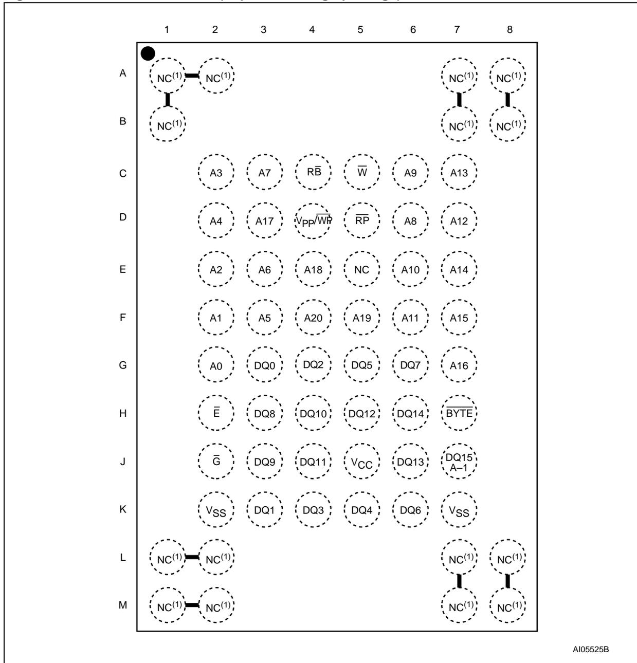
Note: 1. Balls are shorted together via the substrate but not connected to the die.
