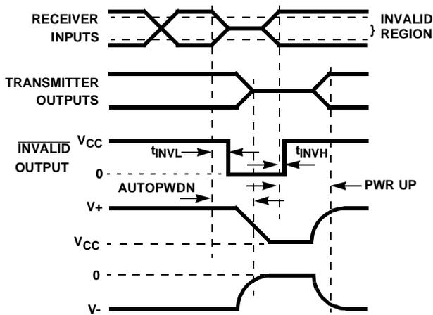
FIGURE 7. AUTOMATIC POWERDOWN AND  $\overline{\text{INVALID}}$  TIMING DIAGRAMS
