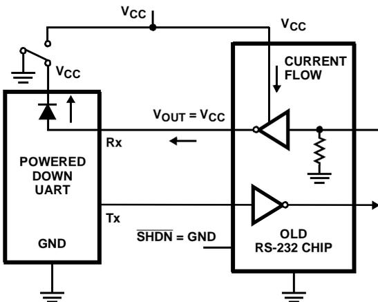
FIGURE 2. POWER DRAIN THROUGH POWERED DOWN PERIPHERAL
